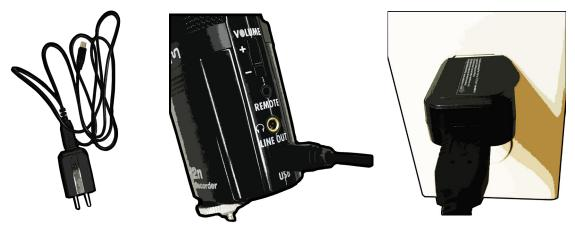
• Plug the H2n Remote into the Remote Control Jack on the left side of the recorder. The remote will allow you to control the recording without touching the recorder.
