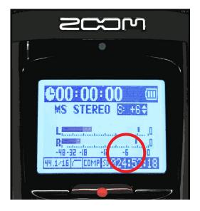
Setting gain too high will pick up more outside noises and lead to distortions in your recording. If the recording seems faint, move the microphone closer to your narrator before increasing gain.
