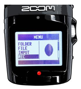
5. On the **REC** menu screen, make sure that **REC FORMAT** is set to **WAV48kHz/24bit**. Press and hold the Menu Button to return to the Home Screen.
