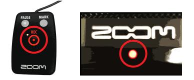
When you need to take a break, adjust your gain, or wish to omit something from the recording, press the PAUSE button; the REC indicator light will begin flashing. Press the pause button again to resume recording. Note: Do not press the REC button to un-pause your recording! This will stop the recording entirely!
